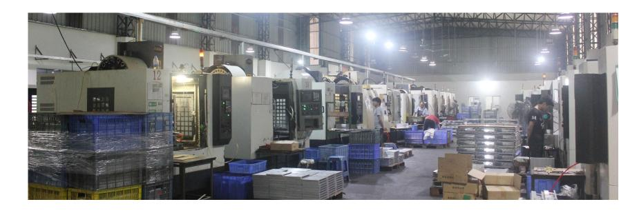
35 sets 3 axis CNC machines, 4 sets 4 axis CNC machines,1 set axis CNC machine
